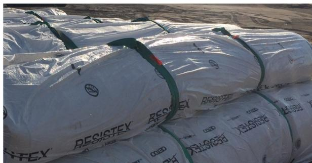
Geosynthetic clay liners (GCL) have long been proven to effectively contain and store municipal solid waste (MSW) while helping maximize space due to their thickness (less than 1 cm), but some experts have taken a closer look at how they perform with special wastes as more operators take in different materials—including coal ash. Mixing coal combustion residuals (CCR) with MSW has raised concerns, especially around leachate compatibility.
